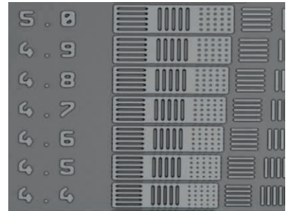
1 μm thick resist with a resolution below 5 μm with a large proximity gap of 30 μm, Source: EVG
