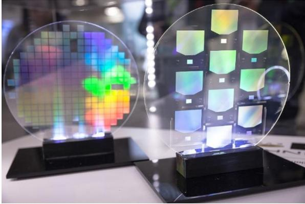
*Figure 1. Nanoimprinted diffractive structures imprinted with EVG tool on SCHOTT substrate using Inkron's high refractive index IOC-resins*
