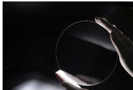
SCHOTT RealView™ glass wafers are made from optical glass with very high refractive index, enabling a wider Field of View (FoV) in AR/MR devices. Image: SCHOTT
