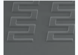
Meander test structures (200 nm)
