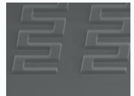
Meander test structures (200 nm)
