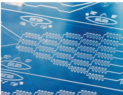
Microfluidic chips replicated in PMMA by hot embossing Source: EVG
