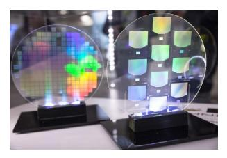
Figure 1. Nanoimprinted diffractive structures imprinted with EVG tool on SCHOTT substrate using Inkron's high refractive index IOC-resins
